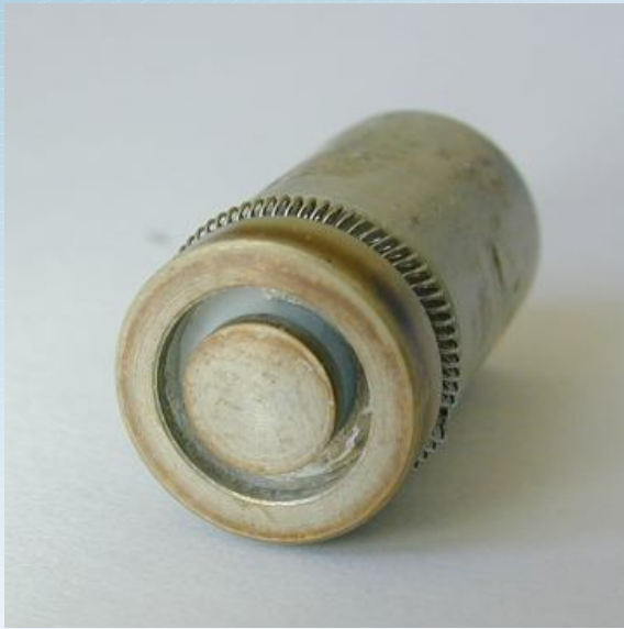
Sensor with PTFE insulator (strongly eroded)
