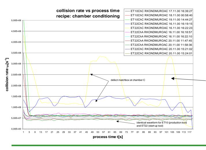
strongly unstable collision rate for conditioning of the chamber
